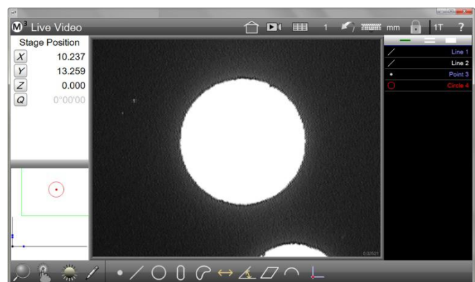
Failed tolerances are shown in red
