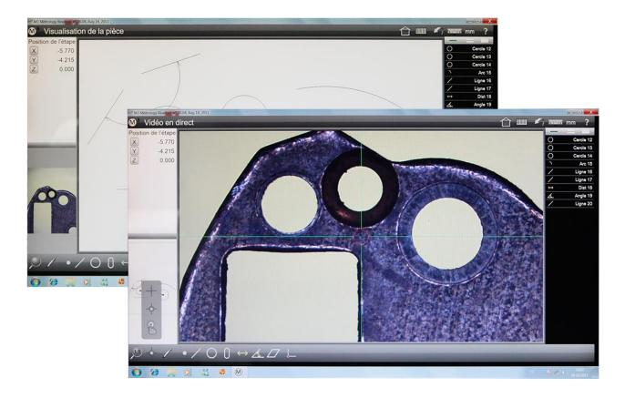
Combined with digital camera, the M3 software is a powerful image analysis system from the last generation which can quickly perform a measurement set.
