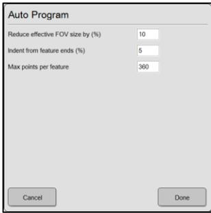
"and program playback will be initiated. Probe the registration features specified on the DXF, directly on the part to be measured. Program playback will proceed once registration is complete.
